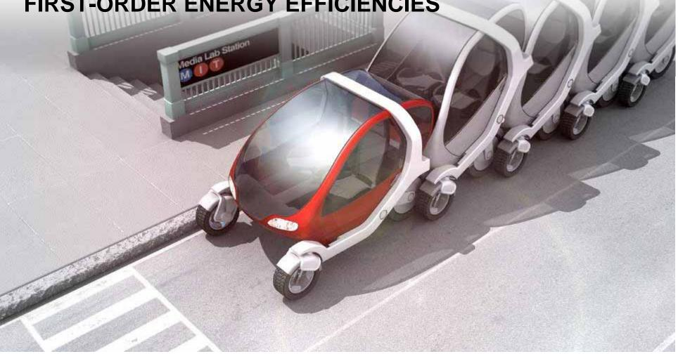
Tiny footprint (size of a Smart when extended, half the size when folded) and much more agile than a traditional car, so makes much more efficient use of urban infrastructure.
