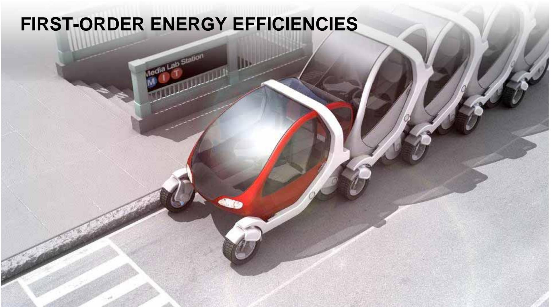
Tiny footprint (size of a Smart when extended, half the size when folded) and much more agile than a traditional car, so makes much more efficient use of urban infrastructure.
